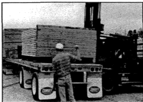
Thousands of square feet of ready-to-install panels can be shipped economically by truck anywhere in the U.S. Panels are loaded with a large forklift equipped with 8-foot long forks. All posts, panels, cants, spikes and freight charges are included in the selling price.
